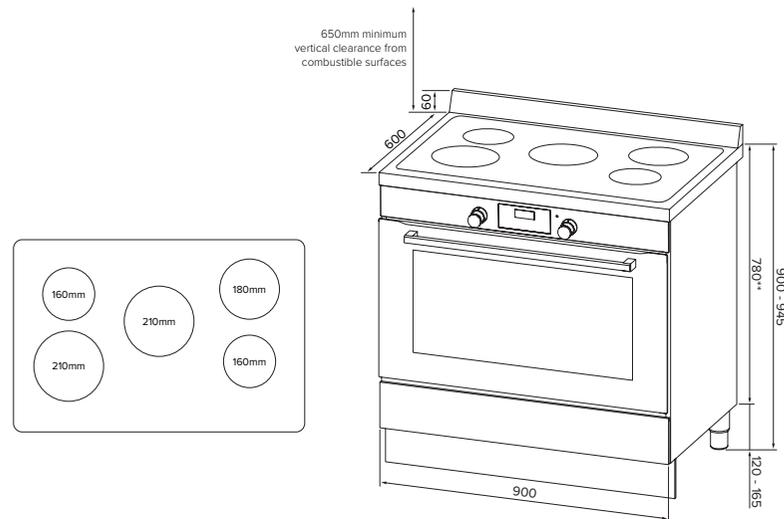
\*\*Height with legs removed for slot in installation on a plinth.
