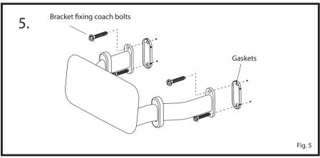
Fit Gaskets onto wall fixing plate as shown in Fig 5. Attach backrest to wall using 4 supplied Bracket fixing coach bolts
