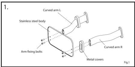
Slide metal covers over curved arms L & R. Attach curved arms to stainless steel body using 4x Arm fixing bolts.
