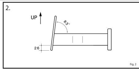
Ensure the angle and the position of stainless steel body is correct as shown Fig 2.
