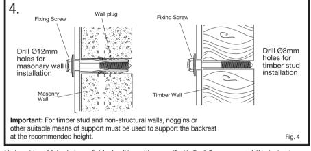
Mark position of fixing holes on finished wall in positions specified in Fig 6. Ensure correct drill hole sizes is selected for timber or masonry installation as specified in Fig 4.
