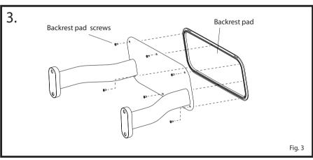
Attach backrest pad using  $6\ x$  backrest pad screws as shown in Fig. 3. Ensure all screws are started before tightening. Do not overtighten.
