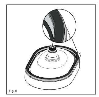
**4.** After ensuring the underside surface of the dress ring is clean then apply thick and wider bead of silicone on the bottom face, as shown in **Fig. 6**. **IMPORTANT:** There should be no open areas on the silicone bead to ensure a water tight seal with the bench.
