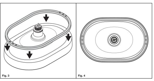
2. Follow the waste assembly instructions and fit the waste assembly, Ensure waste threads and nut are watertight on the underside of the basin waste. Determine which side the CAROMA logo is and by keeping that side towards the back, place the basin upside down and clean the fitting face of the basin which comes in contact with the dress ring to ensure its free of dust, dirt and grease.
