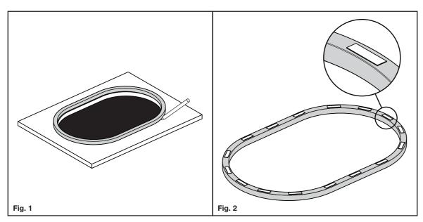
1. Follow the basin cut-out template to cut the bench cut-out.
