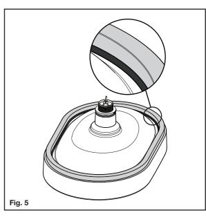
**3.** Apply thick bead of silicone to the inside of dress ring, as shown in **Fig. 5**, smooth the caulking down gently along the joint line using the fingers to ensure the silicone has contacted all joint surfaces.
