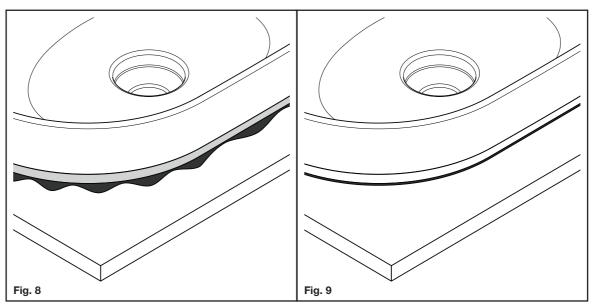
**6.** Connect the trap to the waste assembly, then carefully clean the excess silicone **(Fig. 8)** to achieve a clean joint line, as shown in **Fig. 9**.
