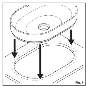
**5.** Flip the basin over and while keeping the "CAROMA" logo towards the back, position the basin onto the bench cut-out by aligning the dress ring with the traced line on the bench, as shown in **Fig. 7**. Push the basin down evenly with both hands.
