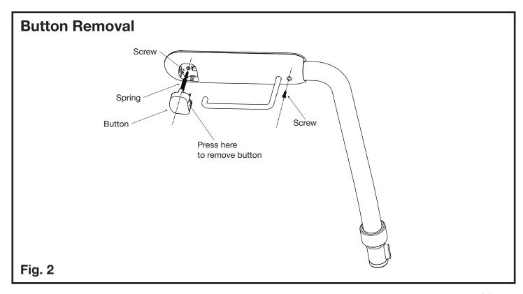
2. Unclip button with small flat bladed screwdriver. Remove button and springs. Remove two (2) phillips head screws.
