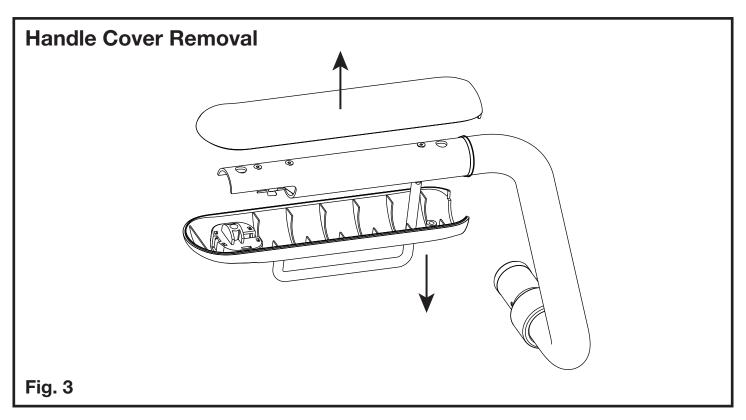
3. Slide lower handle down toilet roll holder. Remove top handle.
