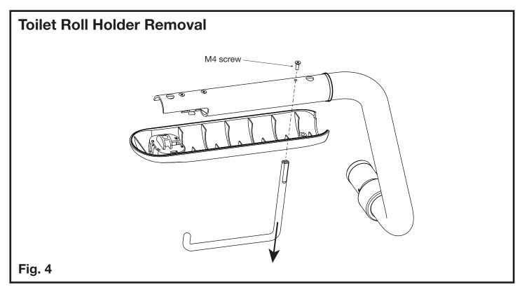
4. Remove M4 phillips head screw and slide out toilet roll holder.
