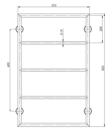
Electricity Input: 240V, 50Hz | Power Rating: 54W | IP Rating: IP55 | Connection position: Bottom right | Connection type: Plug-in only
