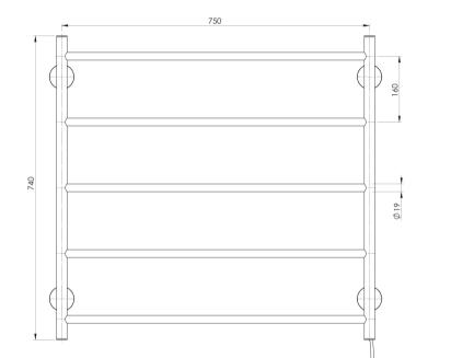
Electricity Input: 240V, 50Hz | Power Rating: 45W | IP Rating: IPX4 | Connection position: Bottom right | Connection type: Plug-in or Hardwire
