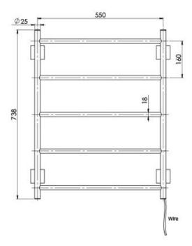
Electricity Input: 240V, 50Hz | Power Rating: 35W | IP Rating: IPX4 | Connection position: Bottom right | Connection type: Plug-in or Hardwire
