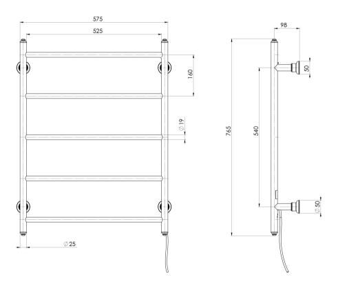
Electricity Input: 240V, 50Hz | Power Rating: 35W | IP Rating: IPX4 | Connection position: Bottom right | Connection type: Plug-in or Hardwire
